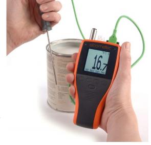
The external sensor of this device type K (TE) has a range of measuring surface temperature from -40 to +200 °C. This device is fully certified, and allowed to use in the territory of the Russian Federation.
