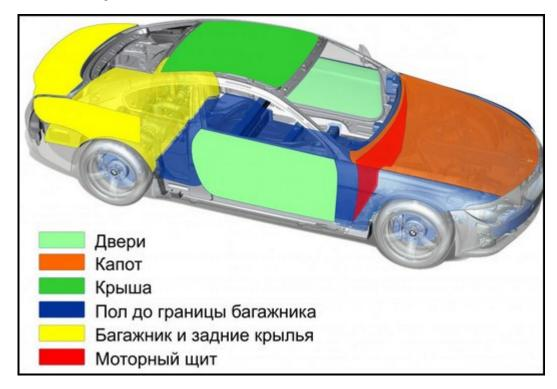
Usually applied self-adhesive foil sound-heat reflectors:
